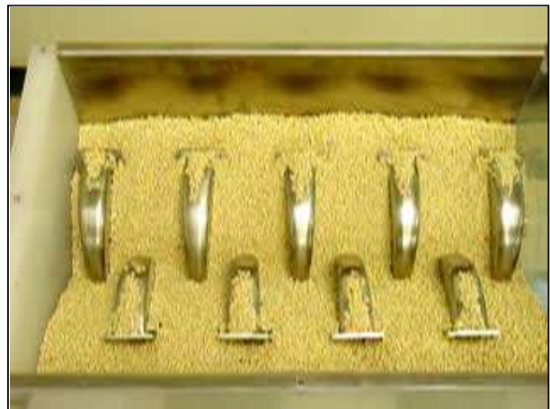
View of a half-filled Hot Paddle Dryer. The paddle shafts use a staggered grip. Optimal mixing and heat transfer.
