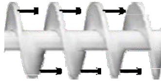
Transport screw: Product contact = heat flow in only a single direction.
